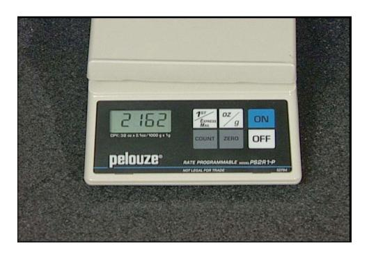
If the new rate chip has been installed correctly the scale will automatically go through its self check operation showing a four digit version code number ...
